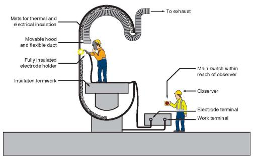
Figure 1: Local Exhaust ventilation in confined space welding
