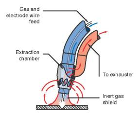
Figure 2: Fume extraction attached to the welding gun
